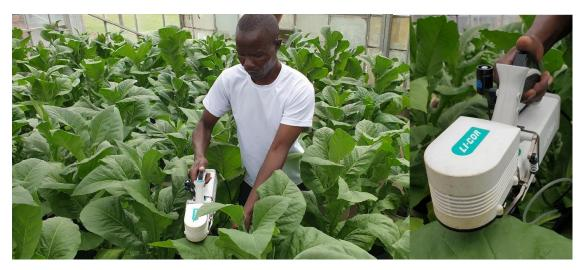
Figure 3: TRB technician using an Infrared Gas Analyzer (IRGA) to take key physiological measurements on the new drought-tolerant tobacco varieties. Photo credit: TRB.
