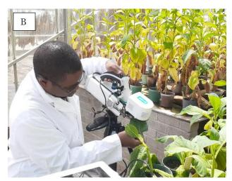
Figure 1: Portable Photosynthesis Instrument (LI6800). A: Key components of the instrument B. Tobacco response to drought experiments in the glasshouse.
