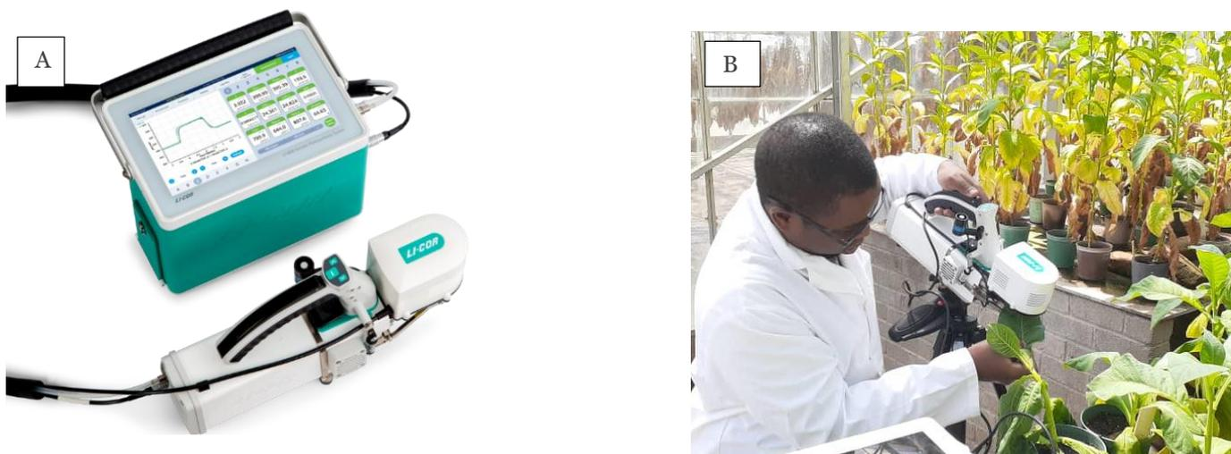
**Figure 1:** Portable Photosynthesis Instrument (LI6800). **A:** Key components of the instrument **B:** Tobacco response to drought experiments in the glasshouse.
