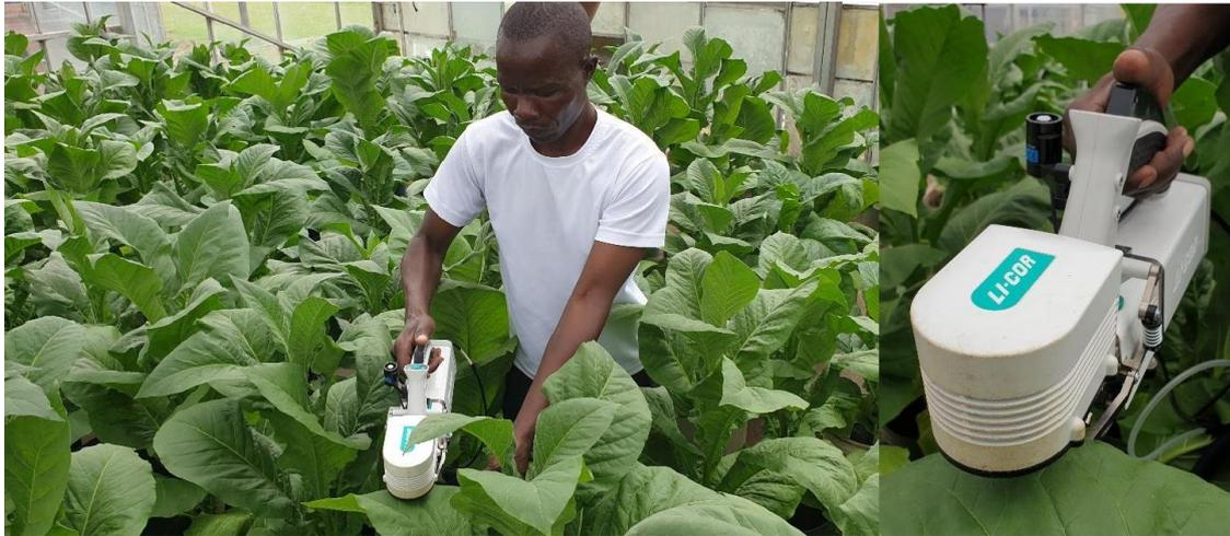
**Figure 3:** TRB technician using an Infrared Gas Analyzer (IRGA) to take key physiological measurements on the new drought-tolerant tobacco varieties. Photo credit: TRB.
